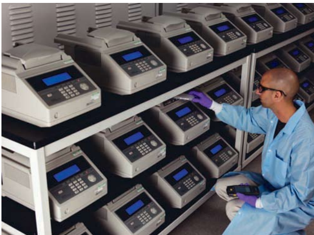
The 9700 system's networking software option lets you control, program, and monitor up to 31 thermal cyclers from a single station.
